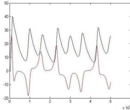
Figure 3: Performance of the 0-1 Test for Detection of Chaotic Chen System.
